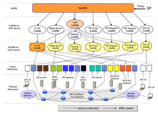
Fig. 4. Autonomic management of VoIP over DiffServ/MPLS.
