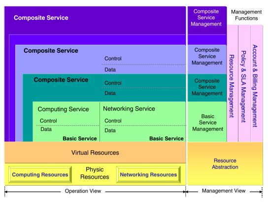
Fig. 1. Autonomic service architecture layered view.
