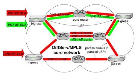
Fig. 6. The path-oriented infrastructure and MPLS trunk deployment.
