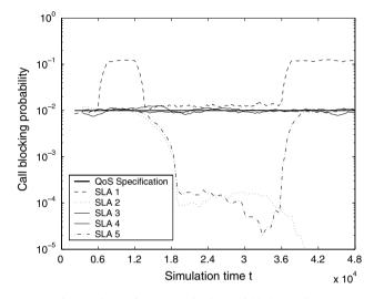
Fig. 8. The performance with bandwidth borrowing.
