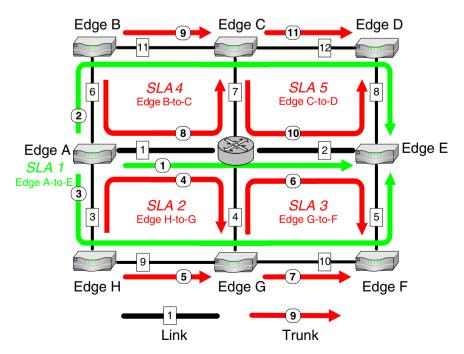
Fig. 7. Network topology, SLA and trunk deployment for simulation.
