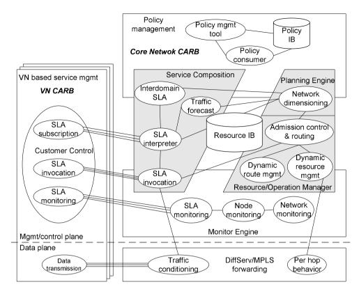
Fig. 5. The CARB for the DiffServ/MPLS core transport network.
