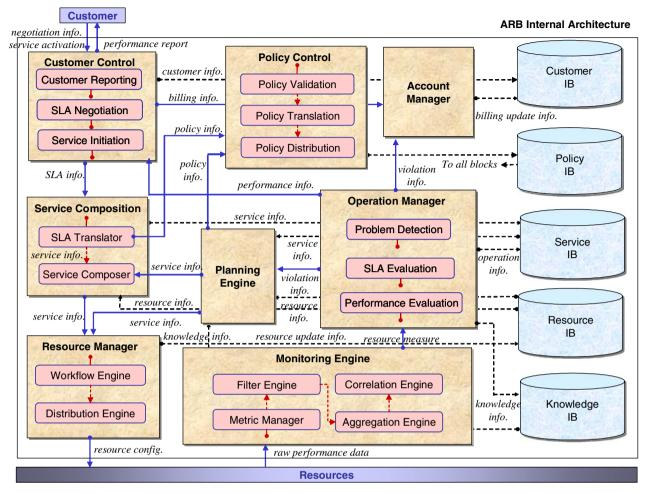
Fig. 3. Autonomic resource broker architecture.
